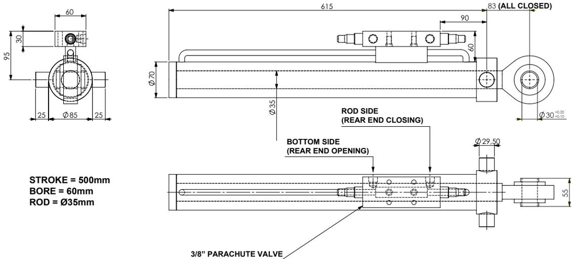
**RIGHT REAR DOOR HYDRAULIC OPENING/CLOSING CYLINDERS FOR TANKS WITH MANUAL LOCKS - STROKE 500 MM**
