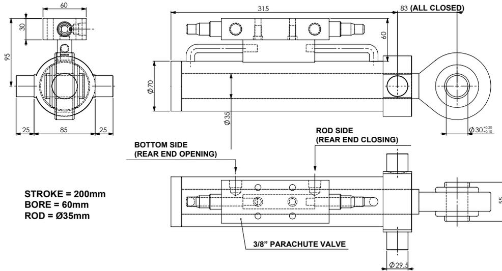
**RIGHT REAR DOOR HYDRAULIC OPENING/CLOSING CYLINDERS FOR TANKS WITH MANUAL LOCKS - STROKE 200 MM**
